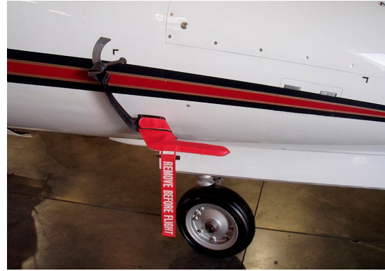
Learjet Heat Resistant Pitot Cover with AOA strap
