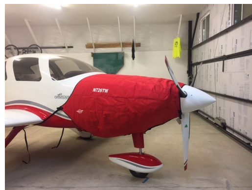
Lancair ES Insulated Engine Cover, Fully Enclosed
