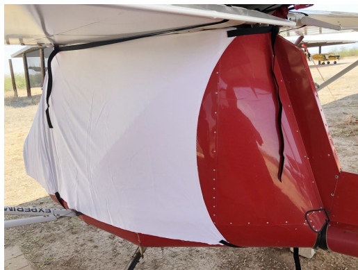
Rans S-12 Airaille Canopy/Nose Cover (test fit cover)
