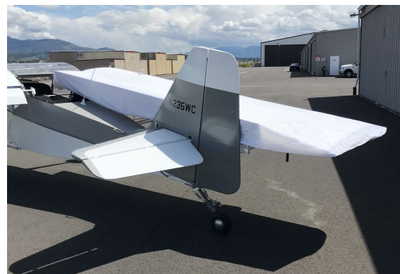
Kitfox Wing Covers, Folded Wing Type, test fit cover
