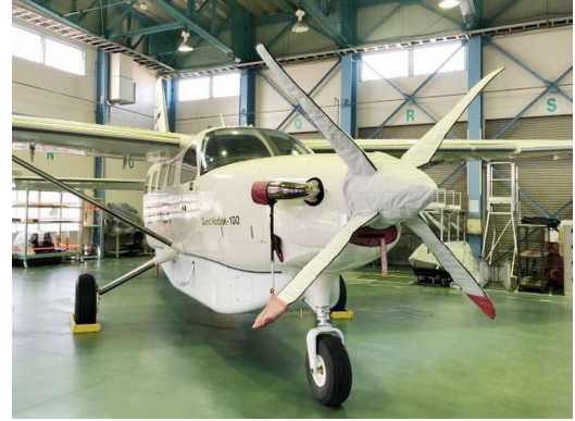
Quest Aircraft Kodiak Insulated Propellor/Spinner Cover, 4 Blade
