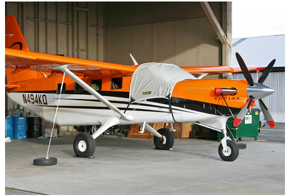
Quest Kodiak Windshield Cover, Prop Tie/Exhaust Covers, Engine Inlet Plugs & Pitot Cover
