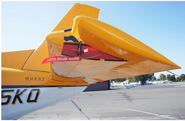
Quest Kodiak Horizontal Stabilizer Lightning Hole Plugs
