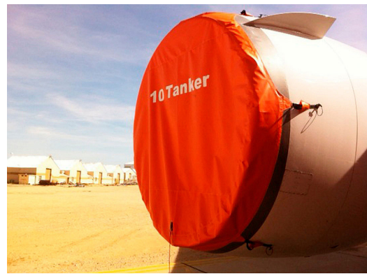
DC-10-30 Intake Cover (CF650C2 Engine)
