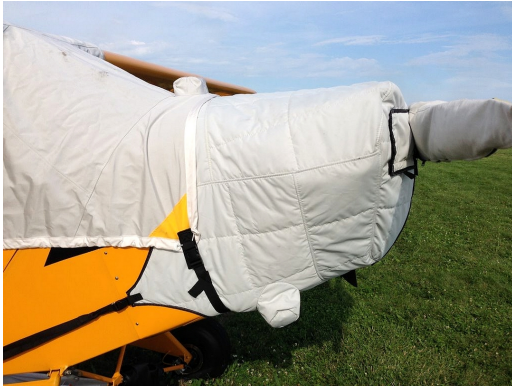
Piper J-3 Cub Insulated Engine Cover with added Pre-heater Access Flaps
