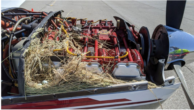
ENGINE PLUGS PREVENT BIRD NEST FOD. Piper Saratoga Engine Cowling Bird's Nest Jabiru J230-SP Engine Inlet Plugs
