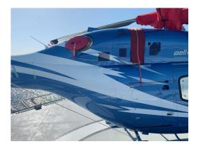
Bell 429 Exhaust Plug, Rotor Mast Cover
