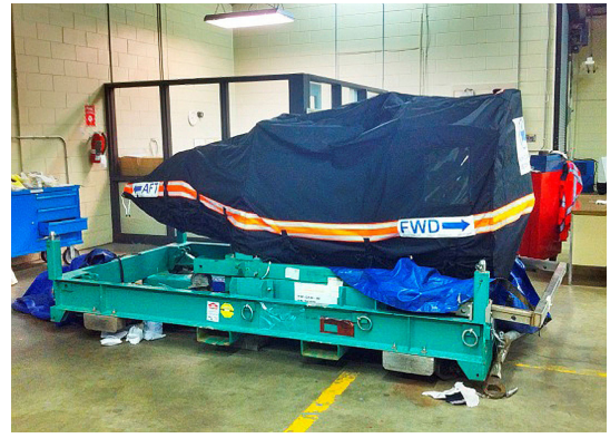
GE CF-34 QEC Engine Long-term Storage/Transport Cover "Bag"
