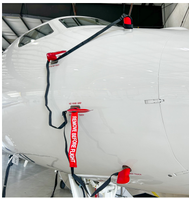
Gulfstream GVII Pitot Probes/TAT/Ice Detector Set, Heat Resistant Type Gulfstream G500 FOD protection plugs for mfg process
