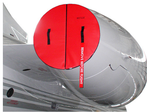
Grumman Gulfstream Exhaust Plugs, folding type
