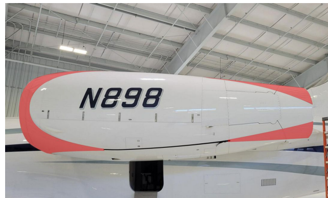
Gulfstream Aerospace G-IV (G350), Intake/Exhaust Cover, test fit cover
