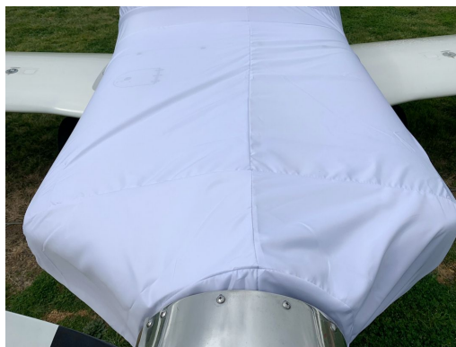
Grob 115 Canopy/Engine Cover, test fit cover
