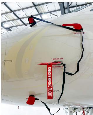
Gulfstream GVII Pitot Probes/TAT/Ice Detector Set, Heat Resistant Type
