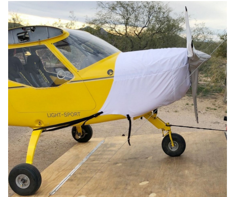
FK-9 Engine Cover, test fit cover
