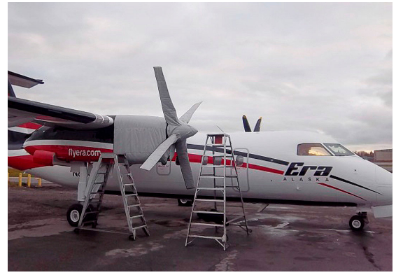
Dash 8 Insulated Engine & Prop Covers
