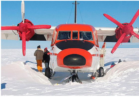
Casa 212 Insulated Engine & Propellor/Spinner Covers
