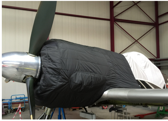
Focke Wulf 190 Canopy Cover & Insulated Engine Cover
