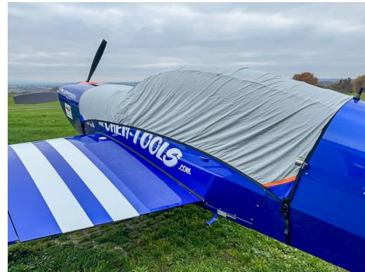
EXTRA 330LT Travel Cover, Light Weight Canopy Cover (2 seat model, Low Wing Models)
