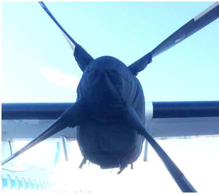
ATR-72-202 Insulated Engine & Prop Hub Covers
