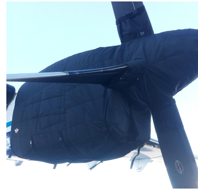
ATR-72-202 Insulated Engine & Prop Hub Covers
