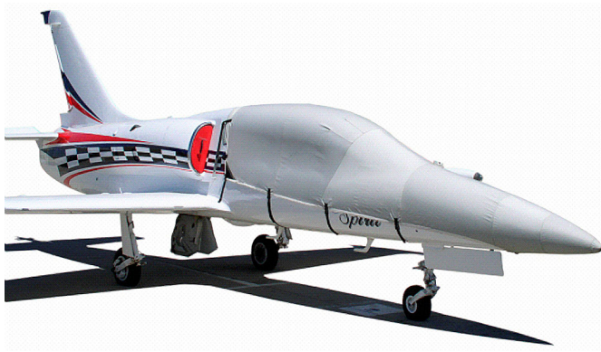
L39 Canopy/Nose Cover & Intake Plugs
