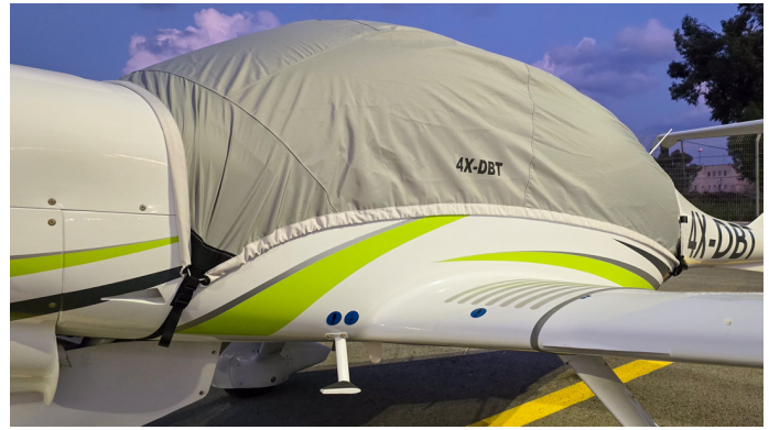
Diamond DA-40 Travel Cover, Light Weight Canopy Cover, Ng Model (Aft Scoop Ext.)
