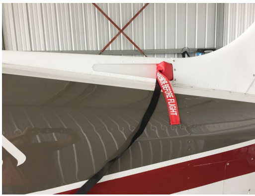
Beech Bonanza/Baron Fresh Air Intake & Exhaust Plugs
