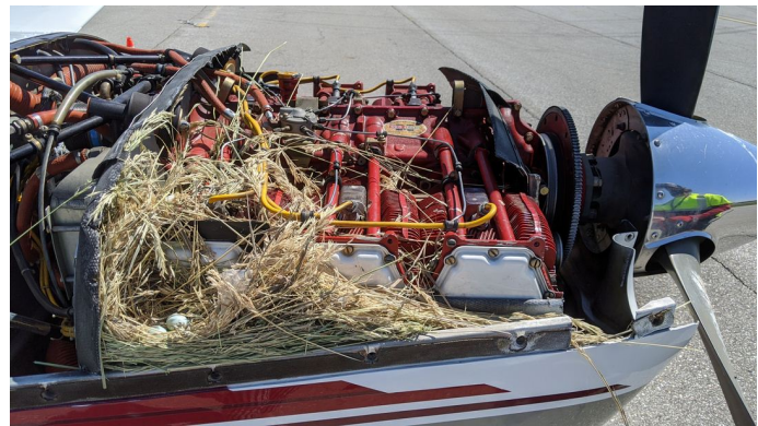
Covers, Plugs & HeatShields for the Dornier 228 ENGINE PLUGS PREVENT BIRD NEST FOD. Piper Saratoga Engine Cowling Bird's Nest
