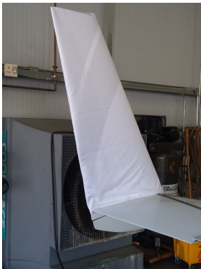
Velocity Vertical Stabilizer Covers, test fit cover
