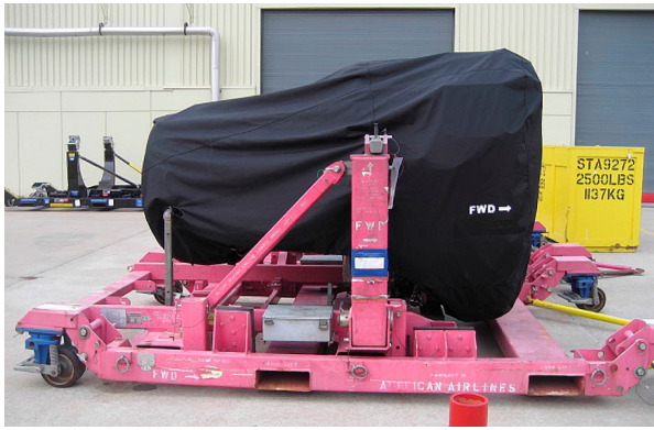
CFM-56-7 Off-link Engine Long-term Storage "Rain Cap" cover, w/o Exhaust Cone, fully enclosed
