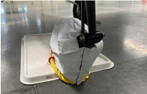
Cub Crafters Tire Covers, tricycle gear, test fit covers
