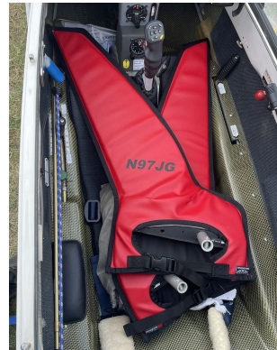
Schempp-Hirth Ventus-2B winglet/wingtip pads
