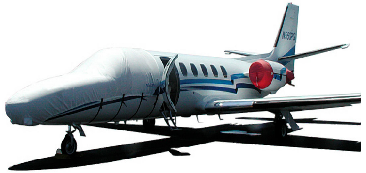
Cessna Citation Nose/Cockpit Cover, Engine Covers
