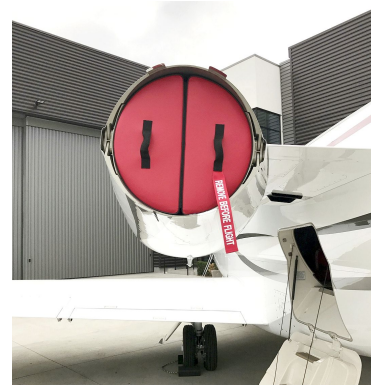
Cessna Citation 680 Exhaust Plugs, folding type
