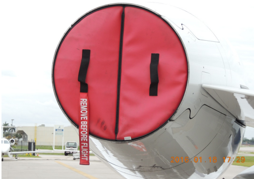
Embraer Legacy 500 Engine Exhaust Plug, folding type
