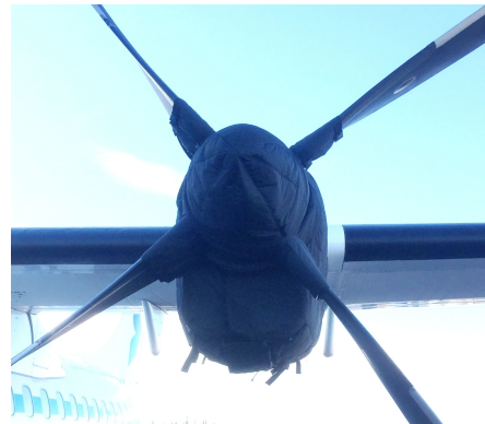
ATR-72-202 Insulated Engine & Prop Hub Covers
