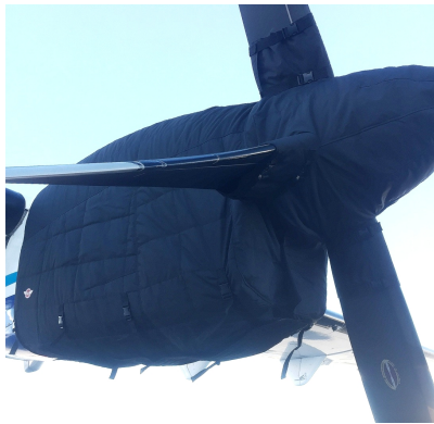
ATR-72-202 Insulated Engine & Prop Hub Covers
