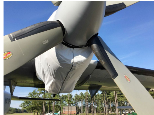
Casa 212 Engine Cover, test fit cover
