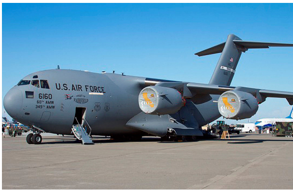
C-17 Engine Intake Covers and Exhaust Covers
