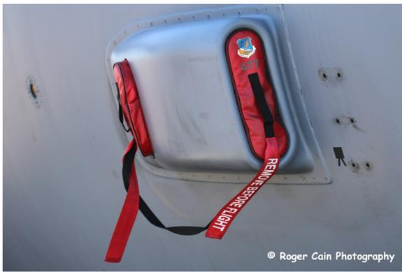
Lockheed C-130 Flight Deck Inlet/Exhaust Plugs
