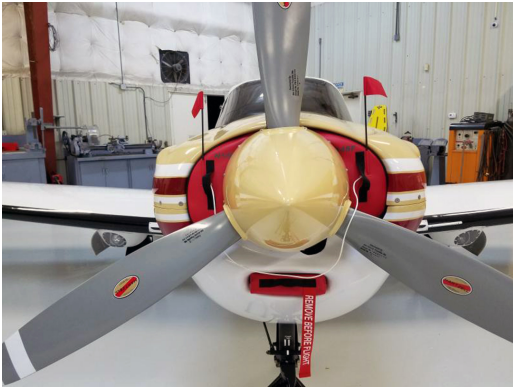
Bellanca Super Viking 17-31A Inlet & Carb Plugs
