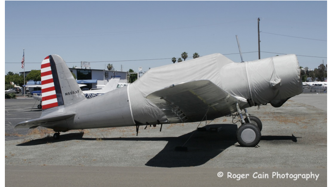
BT-13 Extended Canopy & Engine Covers
