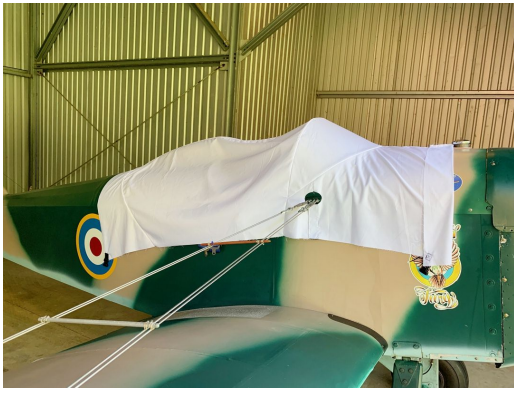
Bowers Flybaby Canopy Cover, test fit design
