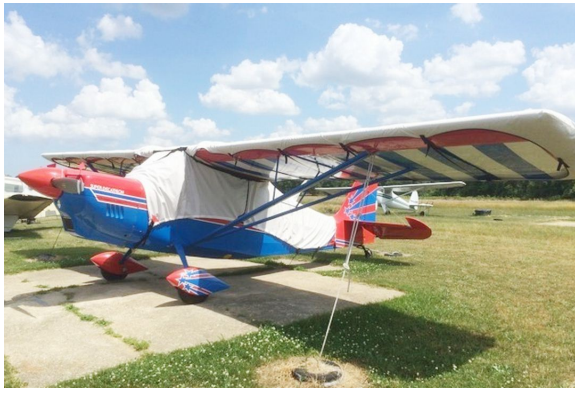
Bellanca Decathlon Canopy Cover (Over-Top, Extended to tail), Wing Covers, Engine Plugs
