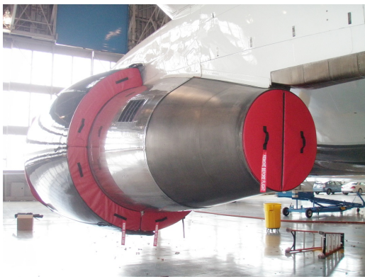
Exhaust Plugs Ship Set, incl. Fan Thrust Reverser and Exhaust Plugs P/N: B767-200
