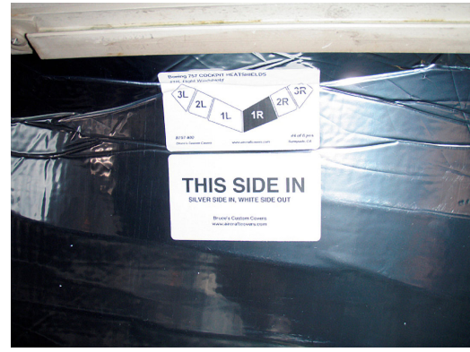
Boeing 757 Cockpit HeatShield set, installation detail
