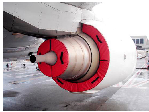
Boeing 737 Bypass and Exhaust Plugs
