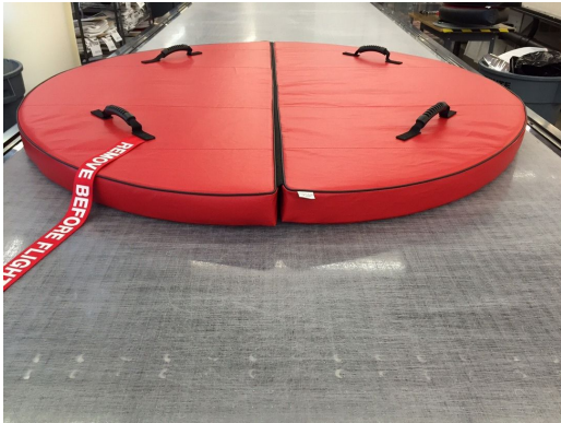
Boeing 737 Max Intake Plug, folding type
