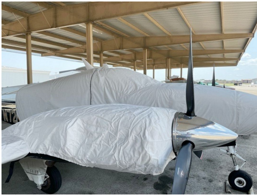
Beech Baron 58P Extended Canopy/Nose Cover, Wing/Engine Covers (test fit) Full Cover Set (58P-020, 58P-225, 58P-405)
