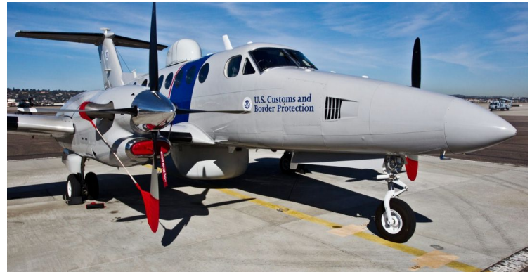
King Air 350 Engine Plugs, Prop Tie/Exhaust Covers
