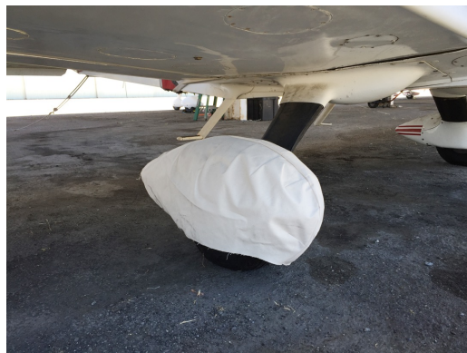
Grumman AA5 Main Wheelpant Cover, test fit
