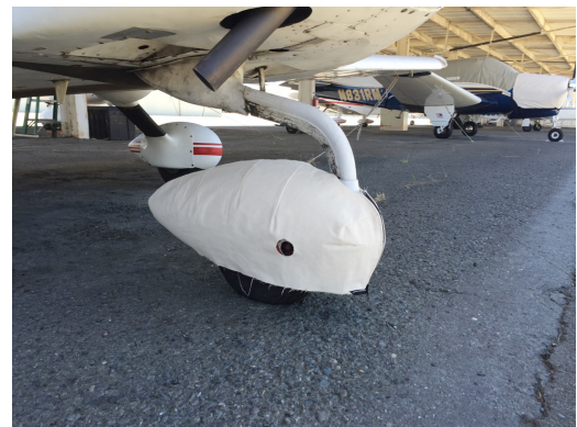
Grumman AA5 Nose Wheelpant Cover, test fit
