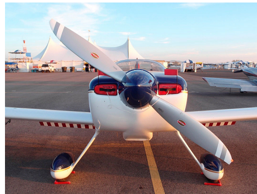
Van's RV-7 Engine Inlet Plugs
