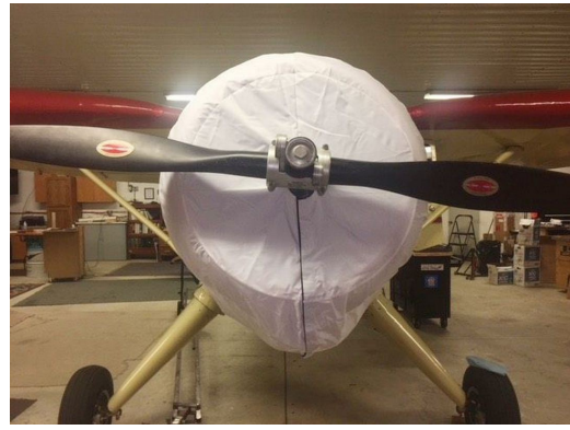
Stinson V77 Insulated Engine Cover, test fit cover
