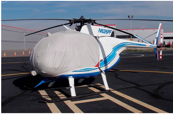
MD500C Bubble Cover with Wire Strike detail
