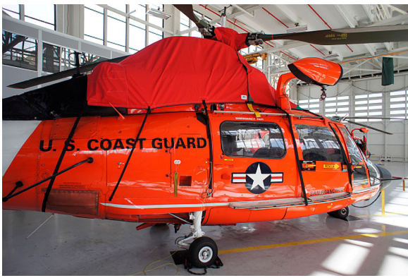
MH-65C Engine Area, Rotor Hub, Swash Plate Aperture Cover set, P/N: A365-210
