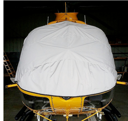
EC-135 Windshield/Skylights Cover, pinches in door jambs
