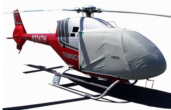
Eurocopter EC-120 Bubble Cover & Tailfan Cover
