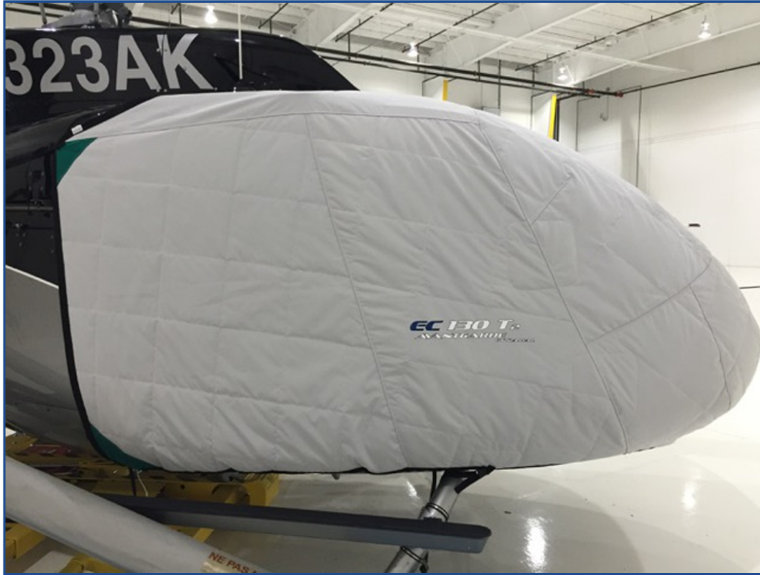
EC-130 Insulated Bubble Cover
