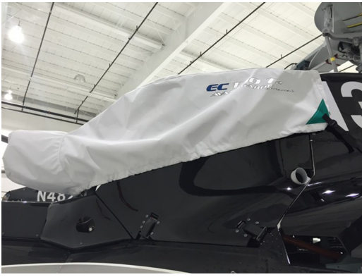
EC-130 Engine Area/Exhaust Cover
