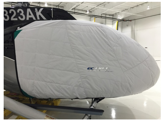
EC-130 Insulated Bubble Cover
