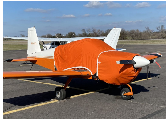
AA-1 Extended Canopy & Fully Enclosed Engine Cover
